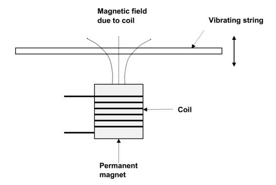
The permanent magnet creates a steady magnetic field near the guitar string. The guitar strings must be made of steel. When the steel guitar string is plucked, an induced EMF (and current) is formed in the coil. This AC electric signal is sent to the loudspeaker to be converted back into mechanical energy.
