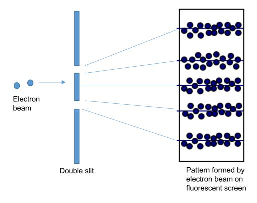
(c) The pattern formed on the fluorescent screen by the electrons as they passed through the double slit one at a time showed evidence that electrons possessed a 'wave nature'. Explain using your knowledge of wave properties.
