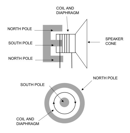
(e) At the instant that the coil is carrying a clockwise conventional current, state whether the magnetic force experienced by the coil is 'into the page' or 'out of the page'.
